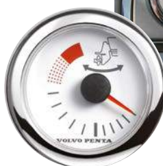
Drive trim position
